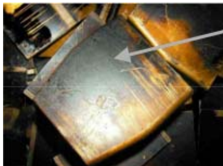
Figure 5: Gas turbine axial bearing pad deposit
